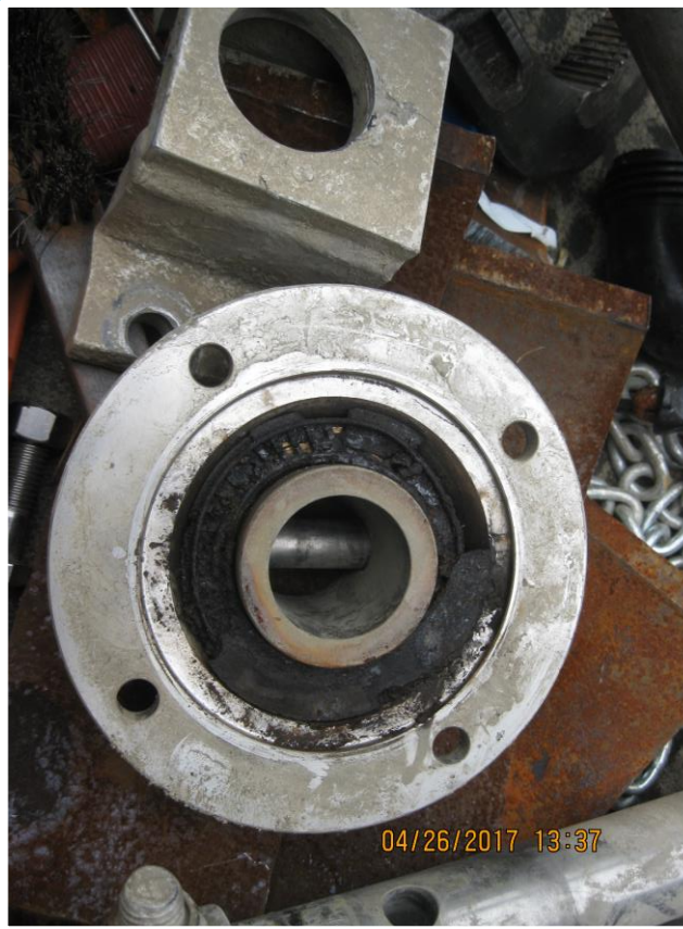
Failed Shaft Bearing from Declez Basin
