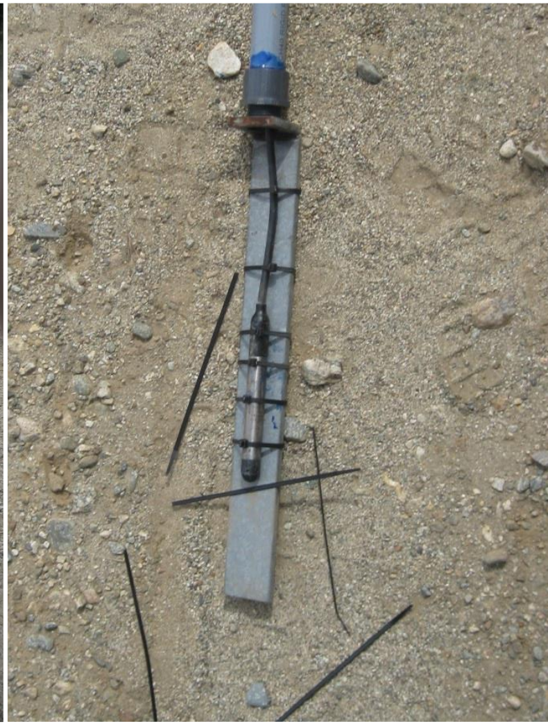
Sled Bracket with Level Transmitter
